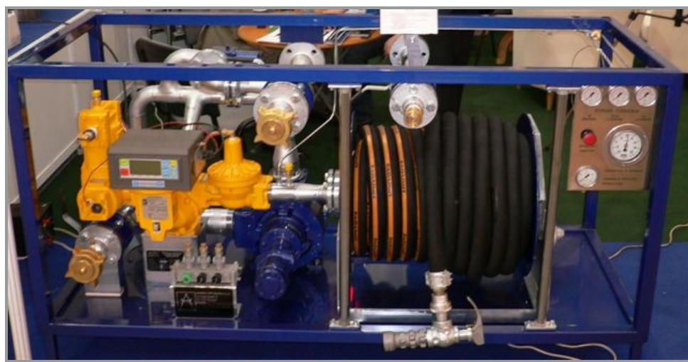
Semi-trailer skid installation with MA7 flow-meter
