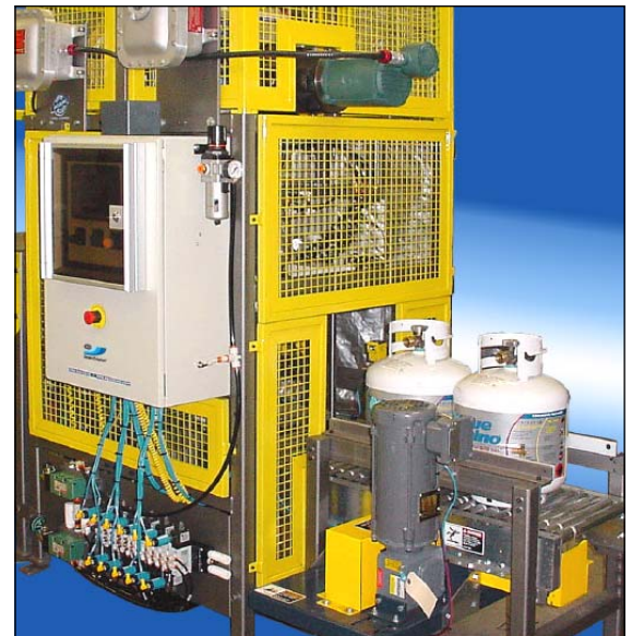
Full-bodied cylinder sleeve application equipment
