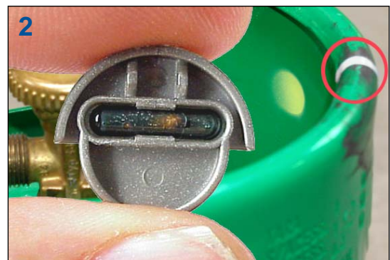
1 & 2 – Examples of cylinder tagging with electronic data carriers
