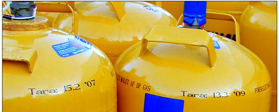
Example of ink-jet printed cylinder data as clear text
